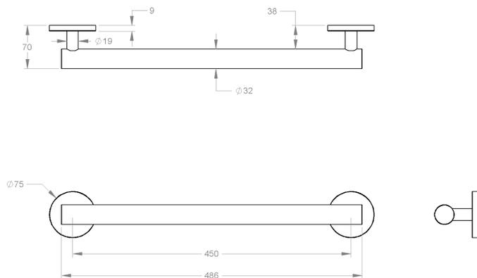
ICO grab bars can support loads of up to 440lbs if properly installed in compliance with ADA requirements.
