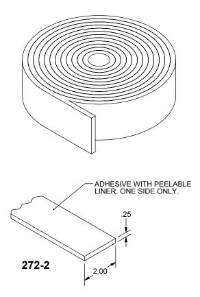
Felt #272-2 HOLDRITE® Isolating felt for use in eliminating dissimilar metal contact and providing sound and vibration isolation. One side is self-adhesive. Available in 25' roll.
