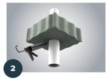
Apply caulking as required to close remaining gap to the bottom side of floor assembly; providing a fire smoke and gas resistant seal. Spread caulking smoothly and evenly all around.
