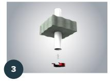
Install collar around pipe from the bottom of floor.
