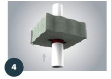
Close collar and slide along the pipe until flush with bottom of floor. Anchors as required.
