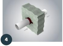
Close collars and slide along the pipe until flush with wall. Anchors as required.
