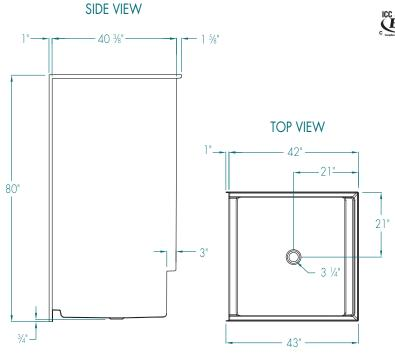
FEATURES Dimensional Tolerance ± %". Dimensions needed for site preparation should be measured from the unit. Manufacturer assumes no responsibility for preparatory work.
