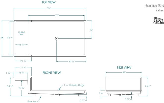
FEATURES Dimensional Tolerance ± 36". Dimensions needed for site preparation should be measured from the unit. Manufacturer assumes no responsibility for preparatory work.
