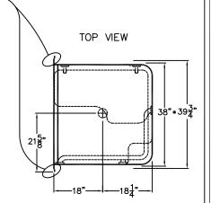
ROUGH IN DIMENSIONS FOR UNITS WITHOUT SEAT FEATURED: 38 1/4" x 37 1/4" x 82 3/4" ROUGH IN DIMENSIONS FOR UNITS FEATURING A MOLDED SEAT: 38 x 37 1/4" x 82 3/4" ROUGH IN DIMENSIONS FOR UNITS FEATURING A FOLD UP SEAT: 39 3/4" x 37 1/4" x 82 3/4" \* NOTE: THIS DIMENSION IS NOT TO SCALE. THIS DIMENSION INCLUDES NUTS/BOLTS, WOOD AND HARDWARE REQUIRED FOR ASSEMBLY. OFFSET THE 39 3/4", 1/2" TOWARDS THE FOLD UP SEAT SIDE TO ALLOW FOR THE BOARD.
