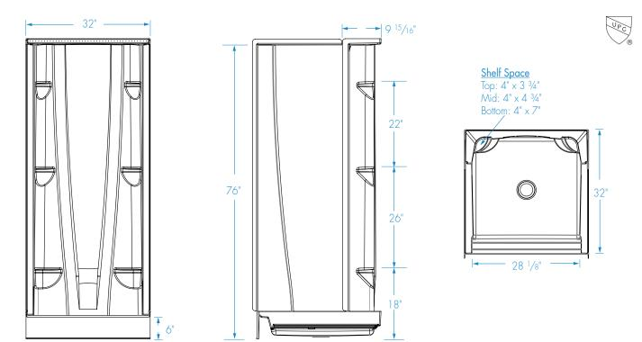
FEATURES Ibs (kg) Dimensional Tolerance ± %". Dimensions needed for site preparation should be measured from the unit. Aquatic assumes no responsibility for preparatory work.
