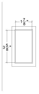
Minimum door thickness required is 1-3/4" when using with pocket lock
