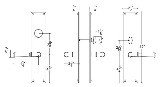
**Mortise Entry** Lock standard backsets are 2-1/2" and 2-3/4" Standard function lock is with emergency egress and various other lock function types are available **Tubular Entry** Latch standard backsets are 2-3/8" and 2-3/4" Standard spacing is 5-1/2" CC and can work with 2-1/8" face bores
