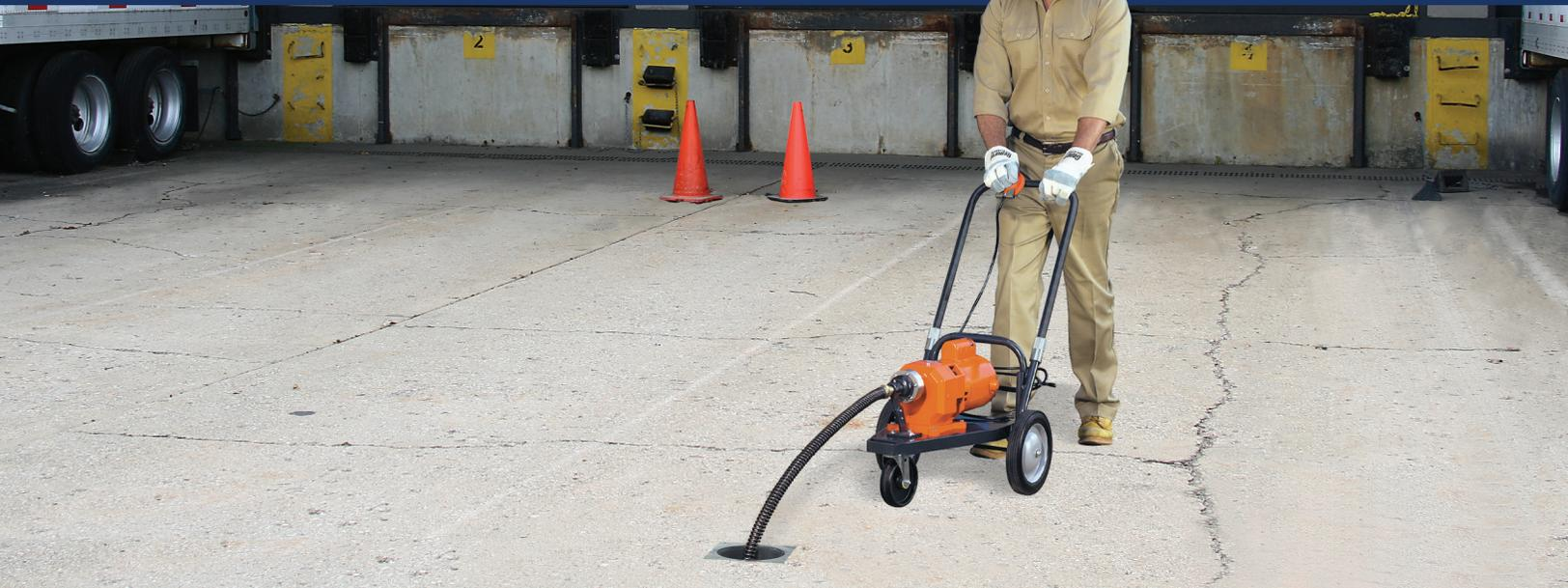
This machine is almost as easy to run as a lawn mower. You push eight or ten foot cable sections into the line until you reach some resistance. Then attach the rear cable coupling to the machine, stand behind it, and turn it on. Watch the cable feed itself into the line. When a section has run into the drain, attach another one and keep going. This self-feeding feature also works to pull sections out of the line.
