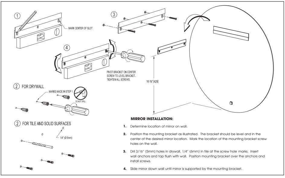
Tools needed: Pencil, Tape measure, Phillips Screwdriver, Drill and Level.
