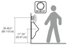
With urinal flush controls a minimum distance of 36" (90 cm) to the opposite wall must be observed to ensure problem-free detection. If urinal flush controls are mounted on opposite walls, a distance of 60" (150 cm) must be observed. Urinal flush controls mounted next to one another must be at least 20" (50 cm) apart.
