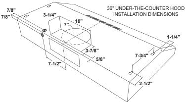
Exhaust outlet connects to  $3\text{-}1/4\text{"} \times 10\text{"}$  rectangular duct. Vent top or rear. Includes rectangular damper.
