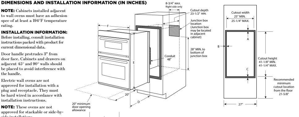
equivalent runners level with bottom of cutout NOTE: If the cabinet does not have a solid bottom and flush with sides of cutout two braces or runners must be installed to support or solid bottom floor. the weight of the oven. For single ovens, the runners and braces must support 200 lbs (91 kg). For double ovens, the runners and braces must support 375 lbs.
