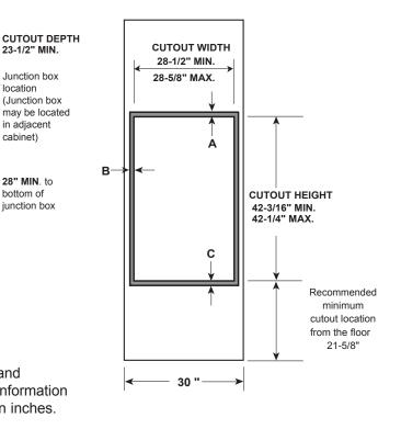
ATTENTION INSTALLER: All electric wall ovens must be hard-wired (direct-wired) nto an approved junction box. A plug and receptacle is NOT permitted on these products
