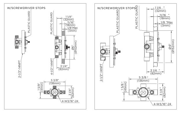
Critical Dimensions : Rough-in valve GS-314-PK (w/stops) & GS-317-PK (w/stops)
