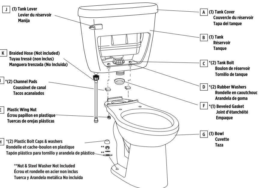
NOTE: Parts with \* are included in tank assembly kit .
