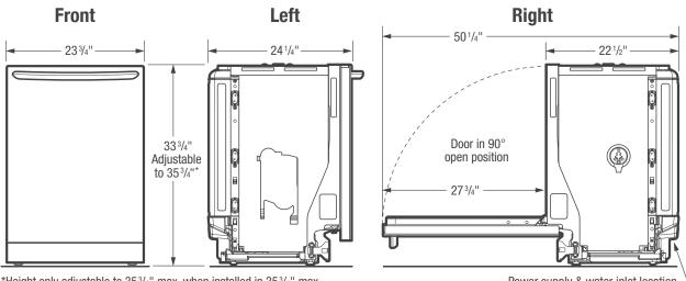
\*Height only adjustable to 353/4" max. when installed in 353/4" max. standard cabinetry cutout. (Dimensions do NOT include insulation – insulation blanket may be compressed during installation.)
