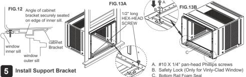
1. Hold each support bracket flush against outside of sill and tight to bottom of cabinet. Mark brackets at top level of sill. Mark cabinet bottom at distance of sill width. See Fig. 15 A. Remove support brackets.
