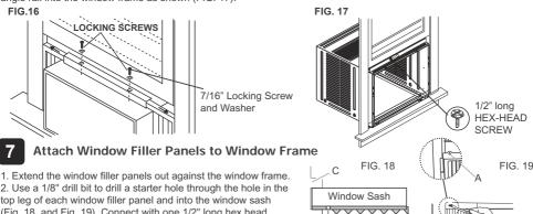
(Fig. 18 and Fig. 19). Connect with one 1/2" long hex head screw.
