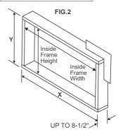
4. Build a wooden frame with the INSIDE dimensions of your model listed above. (Measure twice remember...) Frame depth should be the same as wall thickness. Fill in the space from the opending to the studs with wood spacers, as shown.
