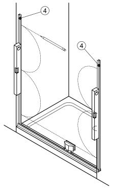
STEP 6: Remove Jamb and drill holes about 1 1/2 deep at each of marked locations .
