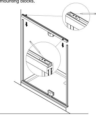
STEP 11: Remove top track and drill holes about 1 1/2 deep at each of marked locations .
