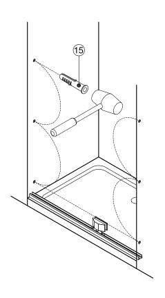
STEP 8: Dab silicone into all 3 holes on each side ,set wall jamb 4 in place and using 1 3/8" screw to attach on the wall.
