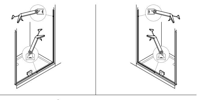
STEP 14: Slide the fixed panel 6 into the caulked wall jamb ,then Adjust the bottom hinge and make sure there is a 22 1/8" wide space for the pivot door.
