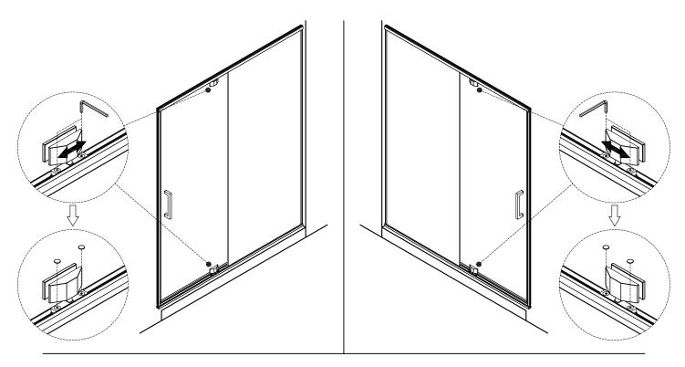
STEP 20: AS Shown ,Cut the track cover ③ to exact size of the door panel and add them over the tracks.
