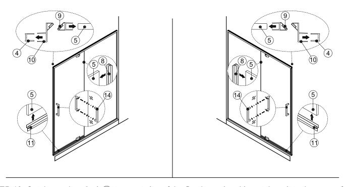
STEP 18: Cut the wedge vinyl  $\bigcirc$  to exact size of the fixed panel and insert them into the gaps of both sides of tracks .
