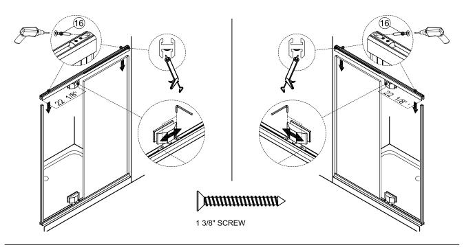
STEP 16: As shown, Install the door panel 5 on the Hinges.
