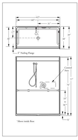
Company. Basic shower will conform to ANSI-Z-124.2. Unit to include stainless steel curtain rod; Symmons® pressure balance mixing valve with concealed check stops; Moen® hand-held shower head with hose and chrome-plated slide bar; stainless steel wrap-around grab bar; stainless steel recessed soap dish.
