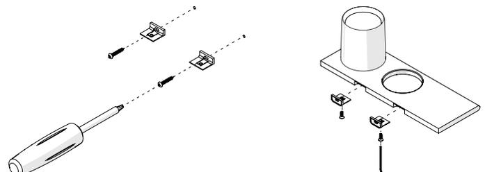
Installer les supports et la tablette / Install the brackets and the shelf
