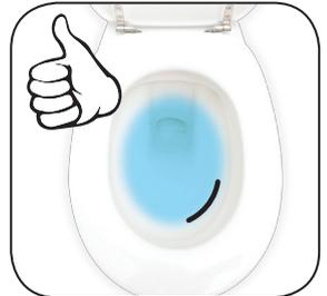
If the water level matches the line in the bowl and the fill valve is **STILL FILLING**, then the bowl water level is **TOO HIGH**, proceed to Step 7D.
