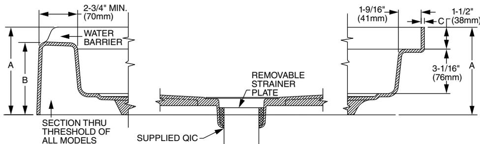
**NOTE:** Quick Drain connector, QDC-2, is supplied with each floor, for use as a drain caulk to replace the lead caulk process (as desired).
