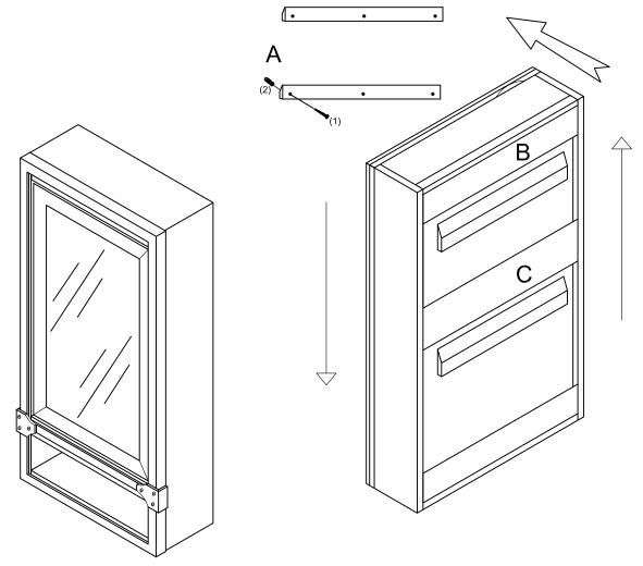
Step 1.Attach the wood cleat (s) A to the wall.
