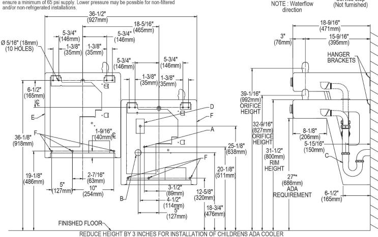
A = Recommended water supply location. Shut off valve (not furnished) to accept 3/8" O.D. unplated copper tube. 3" (76mm) maximum out from wall. B = Recommended location for waste outlet 1-1/2" O.D. drain. Drain stub 2" (51mm) out from wall. C = 1-1/2" Trap not furnished.
