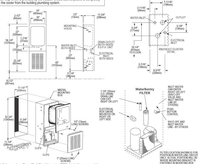
NOTE: New installations must use Ground Fault Circuit Interrupter (GFCI). It is highly recommended that the circuit be dedicated and the load protection be sized for 20 amps.
