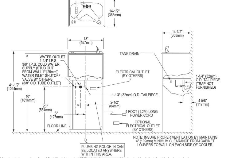
NOTE: New installations must use Ground Fault Circuit Interrupter (GFCI). It is highly recommended that the circuit be dedicated and the load protection be sized for 20 amps.
