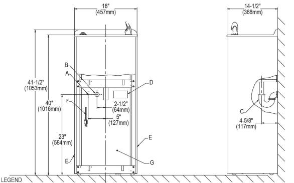
A = Recommended water supply location 3/8" O.D. unplated copper tube connect stub out 1-1/2" (38mm) from wall shut off by others. B = Recommended location for waste outlet 1-1/4" O.D. drain.
