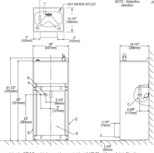
A = Recommended water supply location 3/8" O.D. unplated copper tube connect stub out 1-1/2" (38mm) from wall shut off by others. B = Recommended location for waste outlet 1-1/4" O.D. drain.
