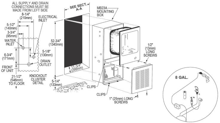
NOTE: New installations must use Ground Fault Circuit Interrupter (GFCI). It is highly recommended that the circuit be dedicated and the load protection be sized for 20 amps.
