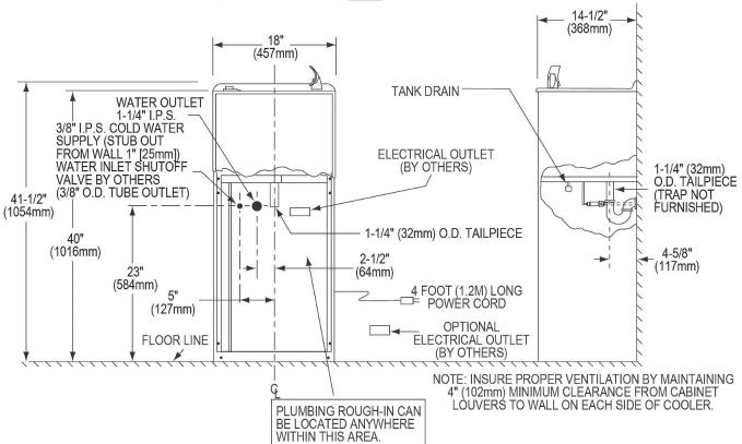
NOTE: New installations must use Ground Fault Circuit Interrupter (GFCI). It is highly recommended that the circuit be dedicated and the load protection be sized for 20 amps.
