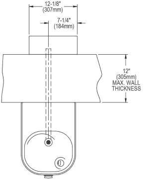
A = Recommended water supply location 3/8" O.D. unplated copper tube connect B = Recommended location for waste outlet 1-1/4" O.D. drain
