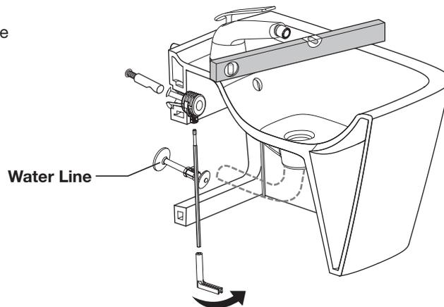
Once bidet is fully mounted into the female threaded nuts, turn the hex allen rod inserted into the plastic housing clockwise to tighten bidet into the finished wall.
