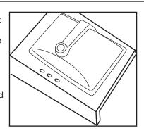
Mount the drain assembly (not included) on the sink, following faucet manufacturer's instructions. Be certain to apply a bead of sealing putty on the underside of the drain (Part "A") in order to ensure a watertight seal between the sink and drain. Remove excess putty after installing drain on sink.
