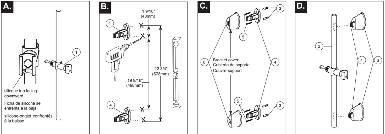
**A.** Make sure the slide mount's (1) silicone tab is facing downward.
