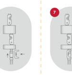
VoicelQ™ Module and secure it with the retaining clip.
