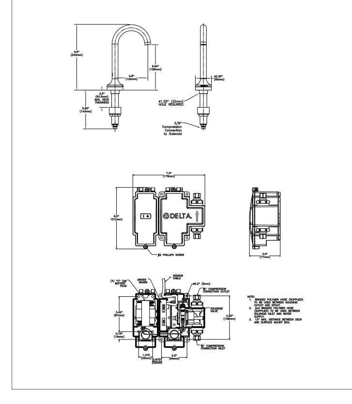
Delta reserves the right (1) to make changes to specifications and materials, and (2) to change or discontinue models, both without notice or obligation. Dimensions are for reference. Measurement may vary plus or minus 6mm(0.25"). Mounting locations are suggested only. Check with local codes for requirements in your area. This spec was produced May 08, 2021.
