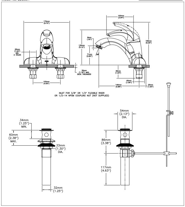
Delta reserves the right (1) to make changes to specifications and materials, and (2) to change or discontinue models, both without notice or obligation. Dimensions are for reference. Measurement may vary plus or minus 6mm(0.25"). Mounting locations are suggested only. Check with local codes for requirements in your area. This spec was produced May 12, 2021.
