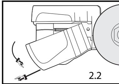
Remove cover by rotating the cover up at the end over the battery compartment and slide out.
