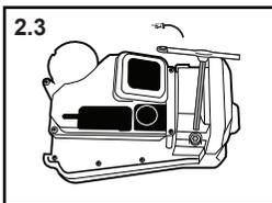
2.1 Remove battery compartment (2.1) and cover (2.2). Using the Allen key, loosen the hex screws and detach the mounting clamp (2.3).
