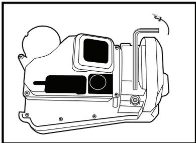
Use the Allen wrench to unscrew the two hex bolts at the neck of the unit until a few threads are still screwed into the connecting bracket.
