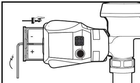
Install 4 "C" cell alkaline batteries into the battery compartment noting the battery position marks on the inside of the compartment. Slide the battery compartment into the Electronic Flush Device unit and secure tray with Allen wrench. The last three turns of the wrench will activate the Electronic Flush Device unit.
