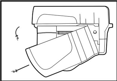
Remove the Electronic Flush Device cover by rotating the cover up at the end over the battery compartment and slide out.
