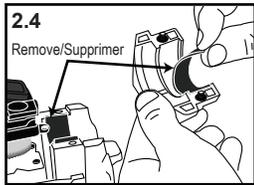
2.4 Remove and discard the existing rubber inserts from the clamp unit.
