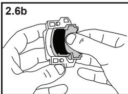
2.6 Place one of the sleeve halves into each side of the mounting clamp.
