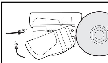
Replace the Electronic Flush Device cover.
