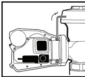
Slide the Electronic Flush Device on to the flush handle and secure the mounting clamp over the existing handle base.
