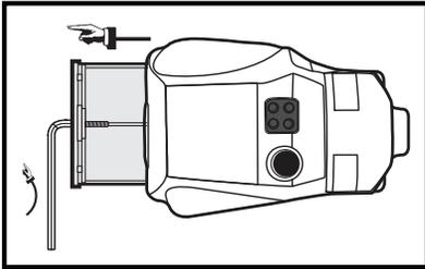
Using the supplied Allen wrench, remove battery compartment.
