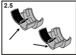
2.5 Place one of the rubber adapter inserts into each half of the grey plastic adapter sleeve.
