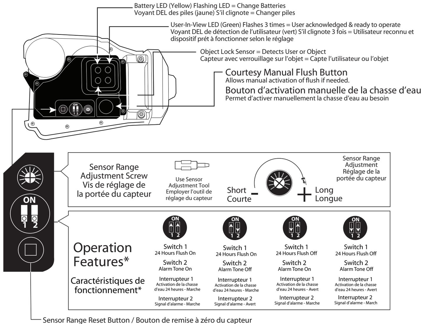
\* Trap Seal Protection (24hr flush): Ensures fixtures are flushed at least once every 24 hours. This feature prevents sewer gases escaping through an open trap. This feature can be turned off by placing switch #1 in the down position.
