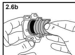
2.6 Place the rear-mounting sleeve half onto the clamp unit. Make sure pin tab of the grey plastic sleeve has been inserted to the mating hole on the clamp unit. Place the front-mounting sleeve half onto the clamp unit. Make sure pin tab of the grey plastic sleeve has been inserted to the mating hole on the clamp unit.
