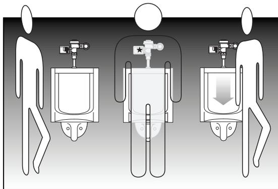
The Electronic Flush Device sends out a continuous infrared beam that is reflected back by the presence of a person in front of the urinal or toilet. "Object Lock" technology differentiates between someone walking past the unit or actually using the fixture.
