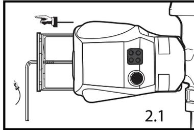
Use Allen Wrench to remove battery compartment tray.
