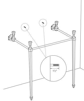
Position the basin on the frame so the hanger bolts extend through the fixing holes.
