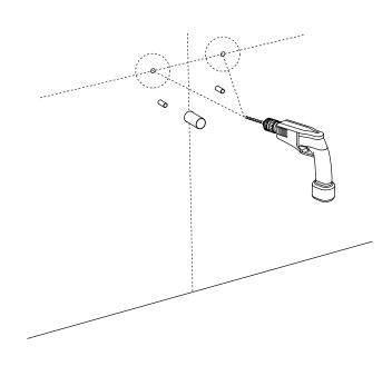
Install hanger bolts so they extend 1-1/2" beyond the finished wall.
