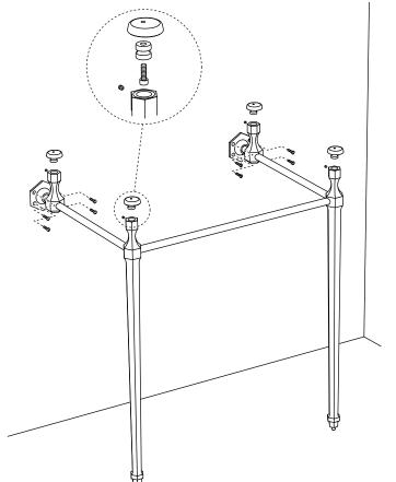
Place the basin in position ensuring that it is level. Mark the basin fixing holes on the finished wall.
