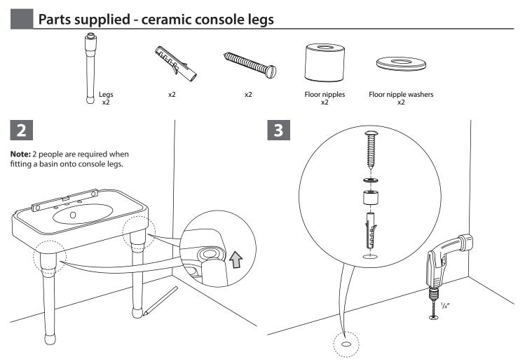
Temporarily mount the basin onto the 2 legs and locate against the wall in the desired position. Once in place, mark the footprint of the leg base onto the floor to confirm the floor fixing position.
