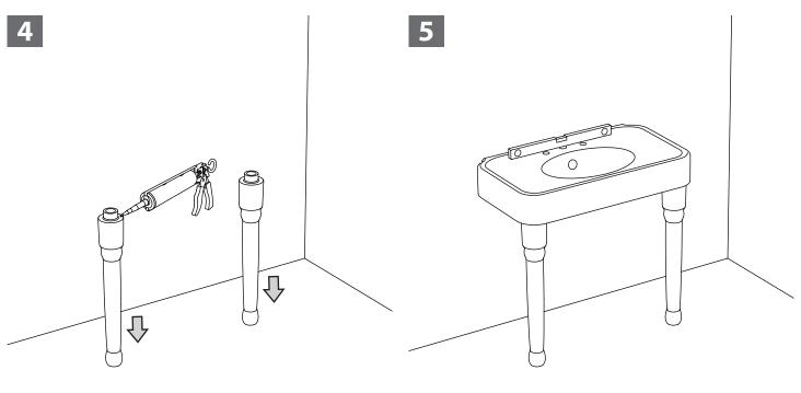
Carefully apply silicone on the top of the legs and then locate the legs over the floor nipples.
