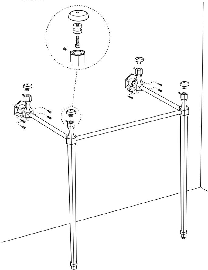
**9** Place the basin in position ensuring that it is level. Mark the basin fixing holes on the finished wall.
