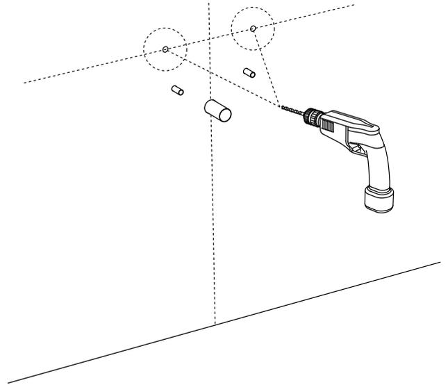
**6** Install hanger bolts so they extend 1-1/2" beyond the finished wall.
