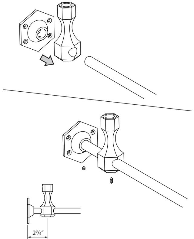
**6** Determine the final installation position and mark the wall fixing hole positions in pencil. Please make sure the frame is level, if required adjust the leg pins.
