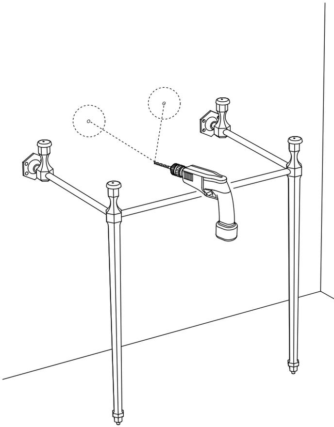
**11** Install hanger bolts so they extend 1-1/2" beyond the finished wall.
