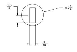
THROUGH-HOLE SPECIFICATIONS RECOMENDED MIN MAXSPOUT: Ø1-1/4" Ø1-1/4" Ø 1-5/8"
