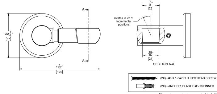
Dimensions are inches, rounded to 1/16" [Dimensions in brackets are mm, rounded to 1mm]
