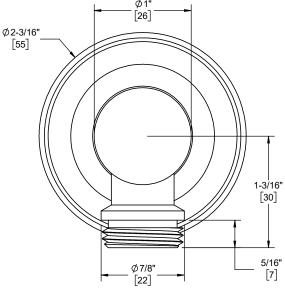
Dimensions are inches, rounded to 1/16" [Dimensions in brackets are mm, rounded to 1mm]
