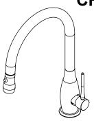
THROUGH-HOLE SPECIFICATIONS MIN RECOMENDED <u>MAX</u> Ø1-3/8" Ø 1-3/8"
