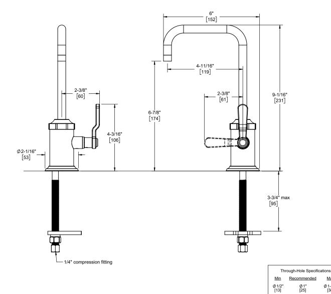
Dimensions are inches, rounded to 1/16" [Dimensions in brackets are mm, rounded to 1mm]
