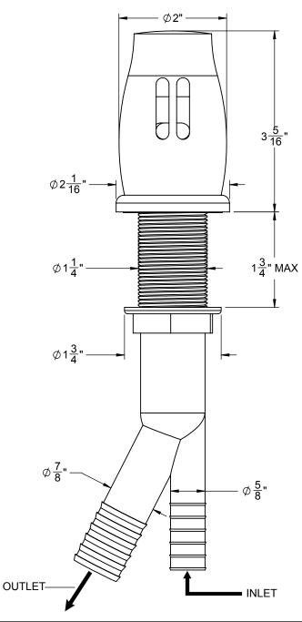
THROUGH-HOLE SPECIFICATIONS RECOMENDED MIN <u>MAX</u> Ø1-1/4" Ø 1-3/8" Ø1-9/16"
