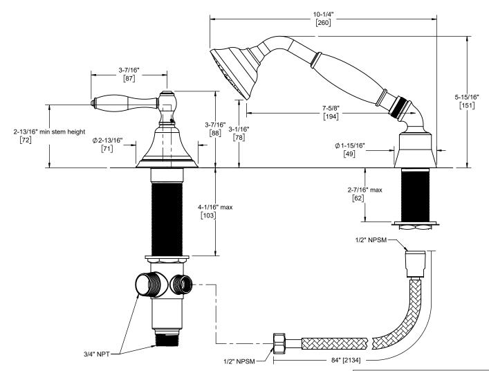
**Through-Hole Specifications** Recommended Shower: Ø1-1/4" [32] Ø1-1/4" [32] Ø1-13/16" [46] Valve: Ø1-7/16" [37] Ø 1-1/2" [38] Ø 1-3/4" [44]
